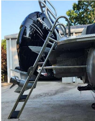
9. If not already installed, attach the (2) ladder snaps to upper section as pictured.
