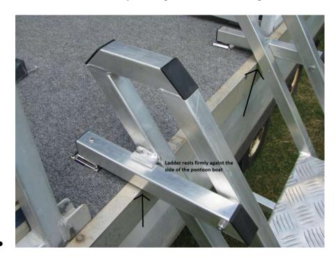
• Next, place the two stainless steel locking keyhole brackets on the ladder nipples and note position on the pontoon deck. Ensure that the ladder is firm against the pontoon boat side. See picture of an installed ladder below:
