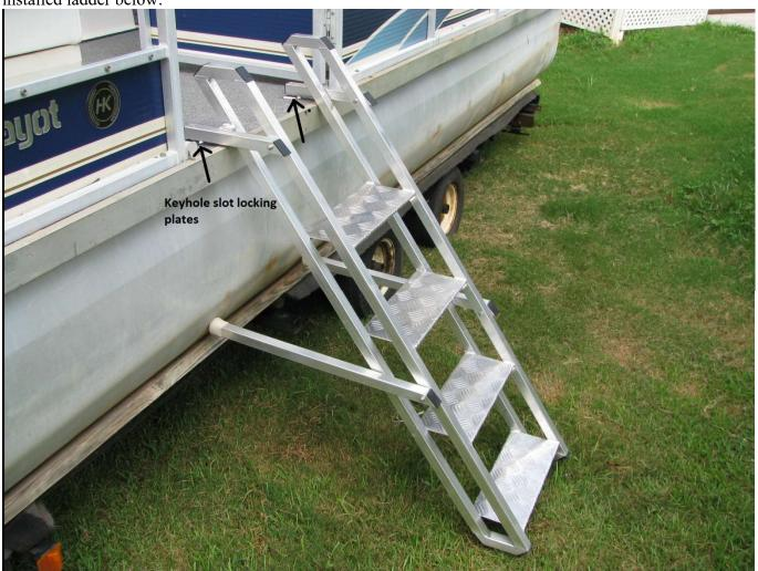
• Secure the locking keyhole slot brackets to deck of boat as pictured:
