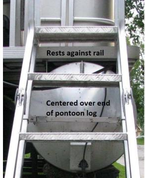
2. Drill two pilot holes through the deck for the two long bolts and place bolts through ladder and deck.
