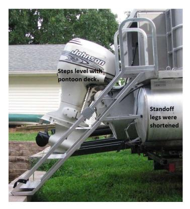
3. Adjust the standoff legs so that the steps are level with the pontoon deck and temporarily install using both standoff legs using two of the short bolts and lock nuts. Make sure beveled end of nylon plugs on the standoff legs match angle of the pontoon log.
