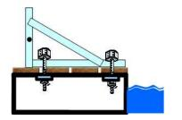
Typical installation of flip-out brackets on wood dock/pier/swim platform. Large galvanized or stainless-steel washers are required underneath the decking to prevent bolts from pulling through surface. The decking itself must be solid and secure. Optionally, a back plate can be used instead of washers.
