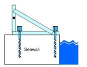
Typical installation of flip-out brackets on seawall. Long galvanized or stainlesssteel lag bolts (or other appropriate concrete anchors) with countersinks into the seawall are required to firmly attach ladder to seawall.
