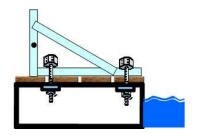
Typical installation of flip-out brackets on wood dock/pier/swim platform. Large galvanized or stainless-steel washers are required underneath the decking to prevent bolts from pulling through surface. The decking itself must be solid and secure. Optionally, a back plate can be used instead of washers.
